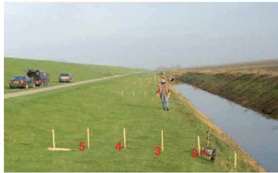
Figure 1 Left: Investigation of embankment with GPR. Right: Resulting radargrams with cavity signatures from muskrats highlighted.
